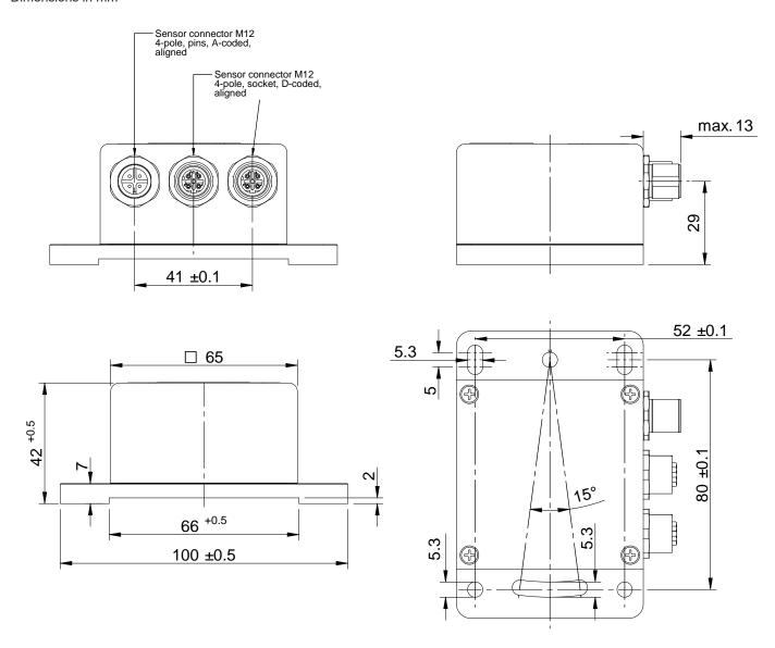
The installation is done via round and slotted mounting holes for M5 bolts. The inclination sensor can be mechanically adjusted up to approx. ± 7.5° via the slots. Fasteners are not enclosed in the scope of delivery. When using the long holes additional security measures must be taken to prevent the device from any accidental displacement.
