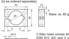
2 Allen head screws M4 x 35 mm (DIN 912, A2) and 2 spring rings (DIN 127, A2) form part of the MB25's scope of delivery.
